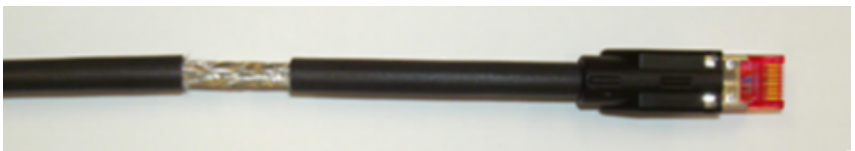
Fig. 10-15: Foil shield removed
