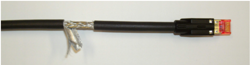
Fig. 10-14: Foil shield of the CDI cable
