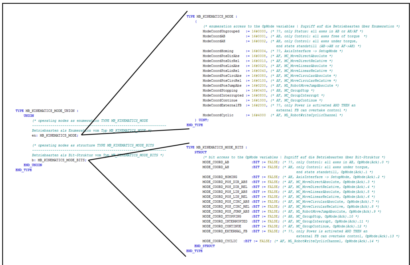
Fig. 18-70: Data type MB_KINEMATICS_MODE_UNION with MB_KINEMATICS_MODE and MB_KINEMATICS_MODE_BITS
