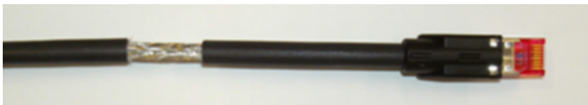
Fig. 10-20: Foil shield removed
